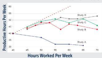
Study A shows productive hours when a person is excessively fatigued. Study B shows productive hours when a person worked four weeks of extended hours. Studies C and D show productive hours when a person worked just one week of extended hours.
